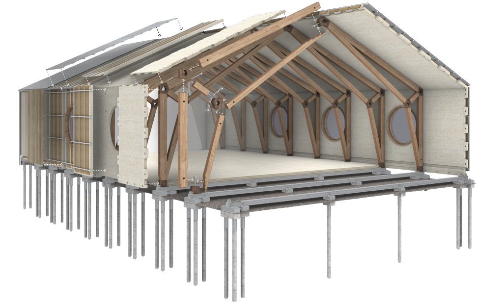
Exterior and disassembly diagram with reusable building elements • 2023 • © Andreas Labes, Berlin / t-lab
